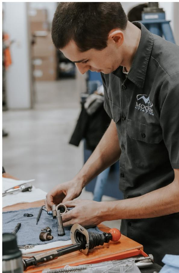
*Ben inspecting hydraulic landing gear pump.*
