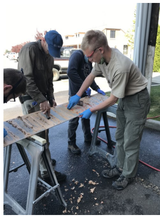
Maintenance Students stripping old paint off an aileron flight control surface
