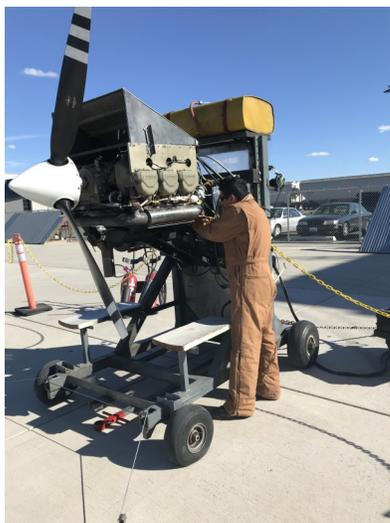
*Running up the turbocharged engine*
