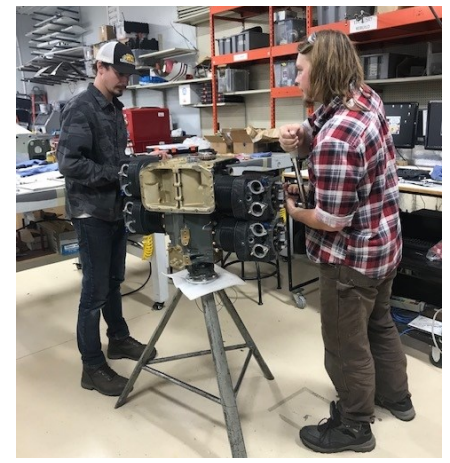
Students assembling an engine that had been completely disassembled and finishing the overhaul process
