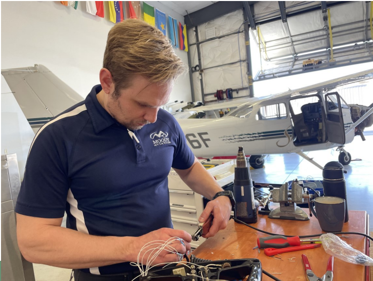
Adding switches to the pilot's control yoke for the autopilot install
