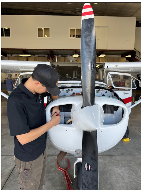
Ben secures an engine cowling after an inspection.
