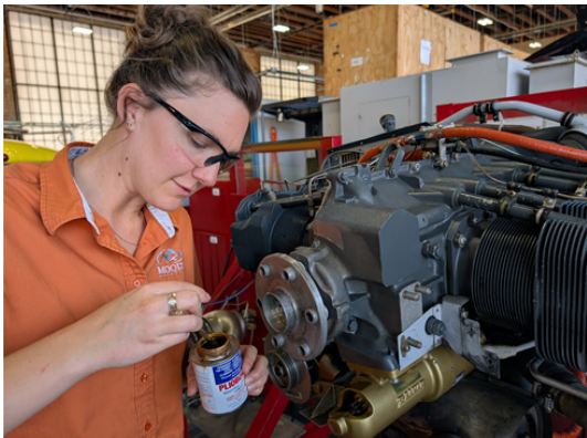
Zoë uses adhesive to install a crankshaft seal on one of Moody Aviation's aircraft engine run stands.
